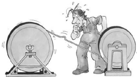
Fig. 6-58b Wrong (rewind the winding)
