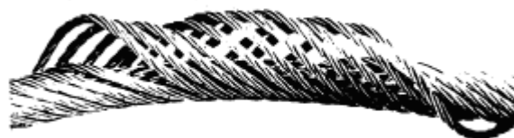
Fig. 6-48 Basket or lantern deformation
